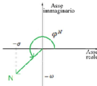
$$N = -\sigma - j\omega \quad \Rightarrow \quad \varphi^N = \arctg\left(\frac{\omega}{\sigma}\right) + \pi$$
